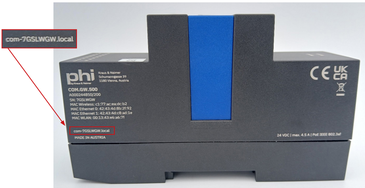
Figure 11: Highlighted in red – the unique DNS address of the COM-Module is located on the left side of the device
